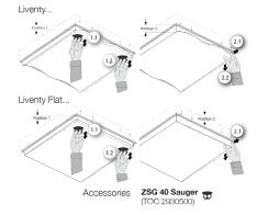
MAKE SURE THAT THE DIFFUSER NOTCHES ARE ALIGNED IDENTICALLY TO THE CORRESPONDING PERFORATIONS IN THE LUMINAIRE BODY
